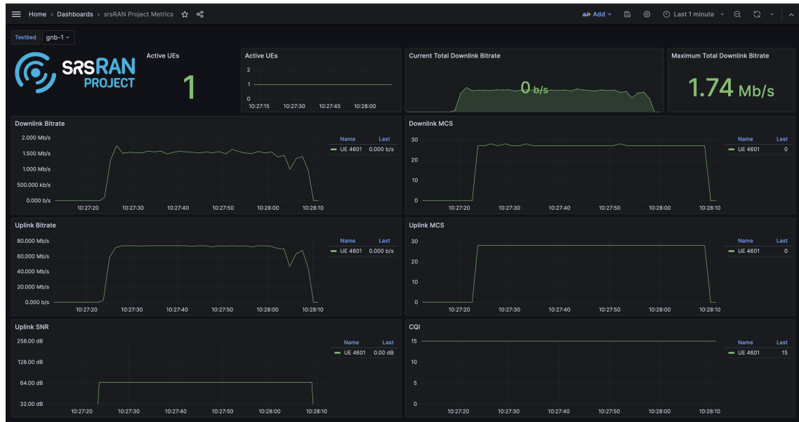
Figure 18 Metrics captured for an iperf3 session from simulated UE to host over virtualized radio. Duration: 45s, max throughput: 100Mbit/s
