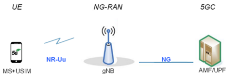
Figure 2.1.: General Architecture 5GS [9]
