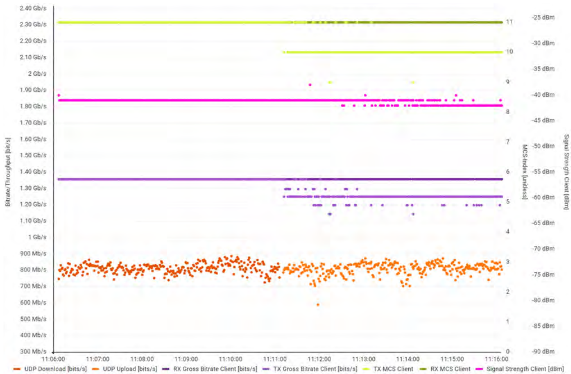
Figure 34: Measurement over 5 GHz with 80 MHz channel width, UDP, between two Clients in two different BSS of an ESS. Throughput reaches 850 Mbit/s which is reduced compared to the 900-1000 Mbit/s reached with an external measurement server.
