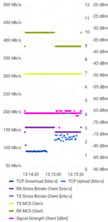
Figure 43: 6 GHz 20 MHz client at 14 m, 23 dBm TP
