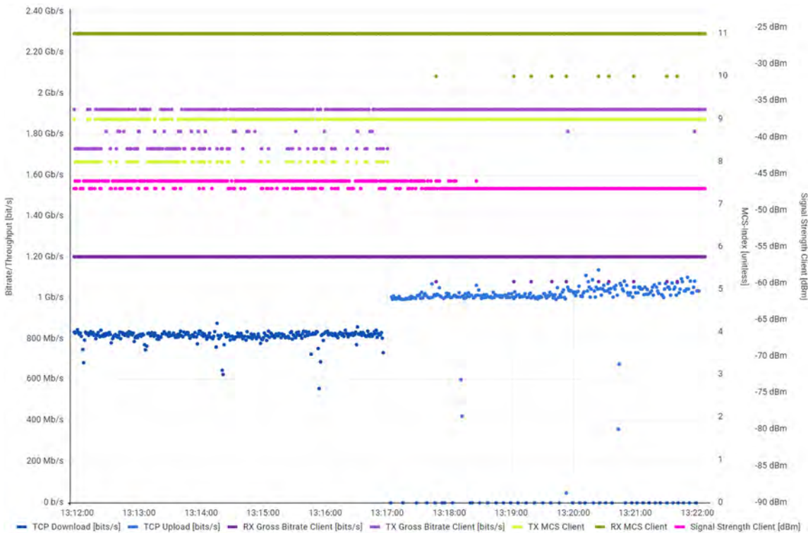
Figure 26: Measurement over 6 GHz with 160 MHz channel width, TCP. Download with one spatial stream, upload with two spatial streams. Throughput reaches over 1 Gbit/s in this case.
