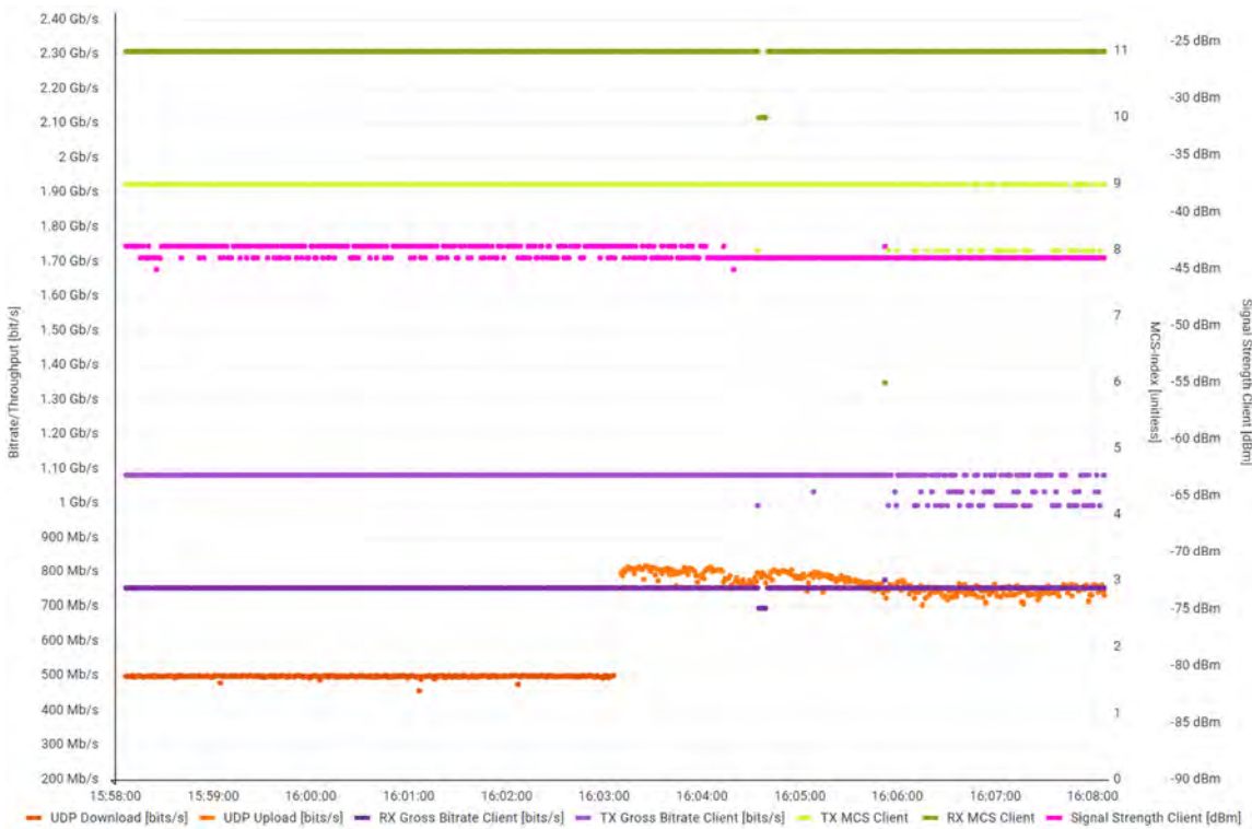
Figure 60: Measurement over 6 GHz with 80 MHz channel width, UDP. Due to only one spatial stream in the download direction download throughput is not directly comparable to download throughput with 5 GHz, which uses two spatial streams.
