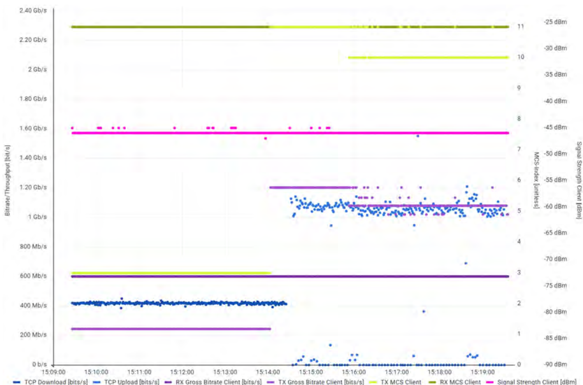
Figure 25: Measurement over 6 GHz with 80 MHz channel width, TCP: Some data points in the upload are zero.
