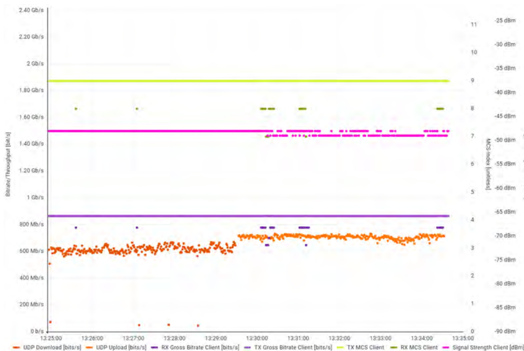
Figure 62: Measurement over 5 GHz with 80 MHz channel width and 802.11ac. Bitrate is lower despite same MCS as in the figure above due to different OFDM characteristics.
